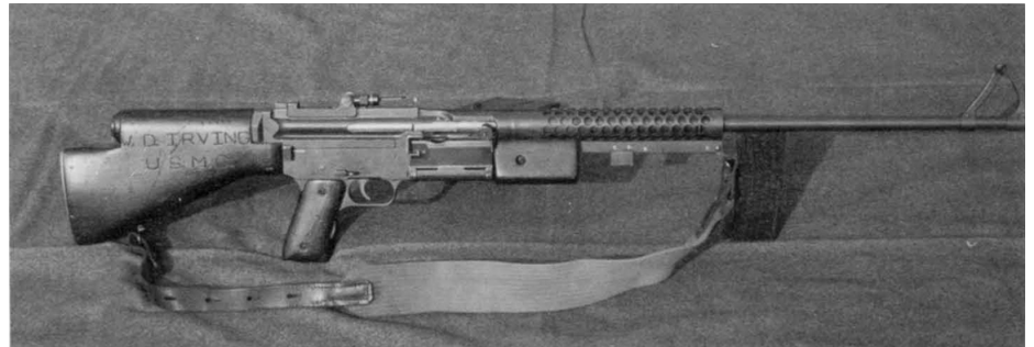
The fully assembled length of the Johnson M1941 light machine gun was 42 inches. It was used during World War II by all three Marine parachute battalions fighting in the Solomon Islands. The parachutists were said to favor the Johnson's buttstock.
